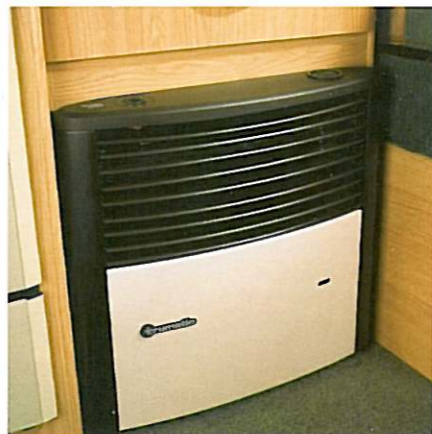
Truma 3002 3kW space heater with Ultraheat ducted blown air heating
