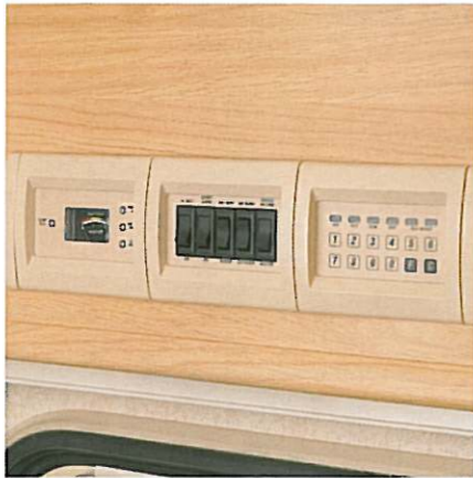
12 volt distribution unit featuring 12 volt isolation and interior entry light switch (GTS Vogue/Spectrum)
