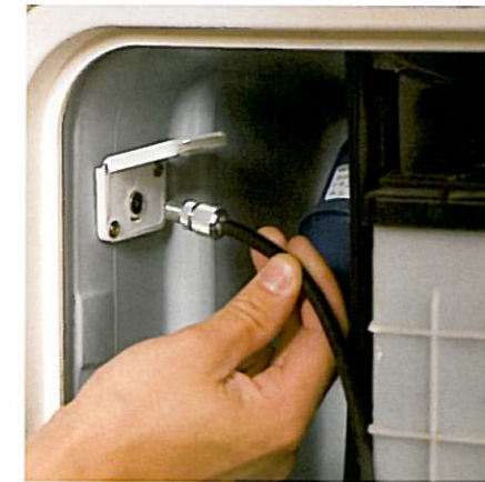
TV aerial socket fitted in battery box for easy connection to site facility
