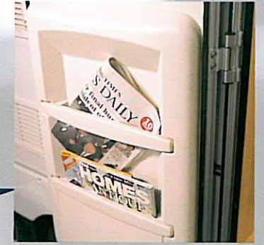
Door liner with integral magazine storage
