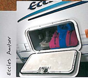
Door liner with integral magazine storage
