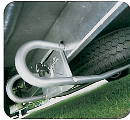
AI-ko spare wheel carrier and spare wheel (Pageant & Senator)
