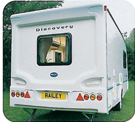
Full height rear ABS panel with integral rear light cluster (Discovery & Ranger)
