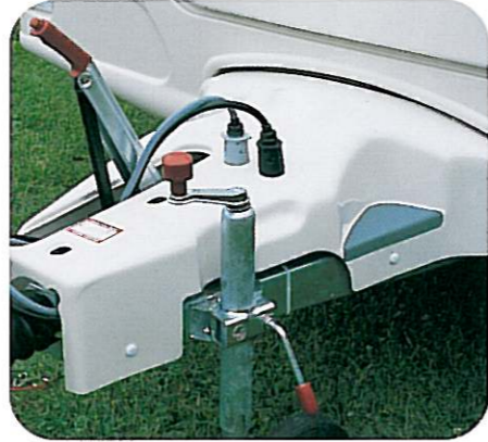
'Step Up' A-frame fairing (Discovery & Ranger)
