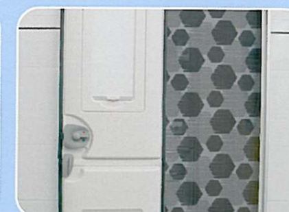
Aircraft style liner for exterior door including storage pocket
