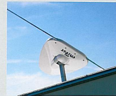
Directional TV/FM aerial and booster
