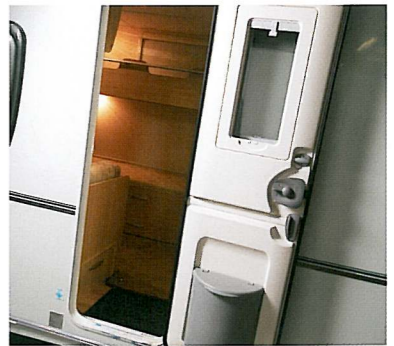
Exterior door with window blind and integrated waste bin
