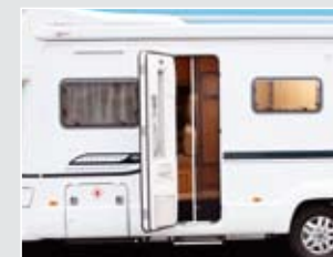
Entrance door New entrance door with secure 3-point locking, hidden hinges, double seal system and stepwell light
