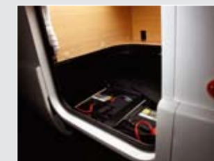
Twin batteries Models now come with two 110Ah auxiliary batteries giving greater independence away from a mains power source
