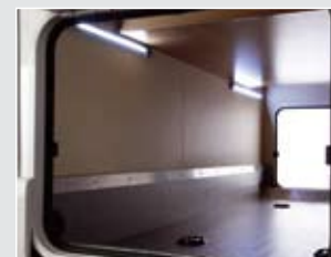
Lighting in underfloor storage trays Underfloor storage trays provided by the Fiat/AL-KO low-line chassis with 190mm (7 1/2") double floor now have lighting in
