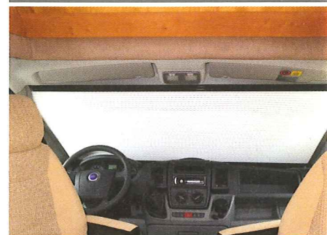
Windscreen and bays with insulating blinds
