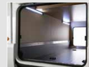
Lighting in underfloor storage trays Underfloor storage trays provided by the Fiat/AL-KO low-line chassis with 190mm (7½") double floor have lighting
