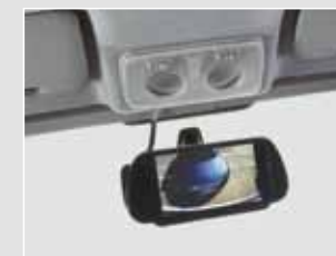
Reversing Camera Reversing camera with image shown on rear view mirror
