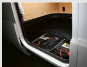
Twin batteries Models come with two 100Ah auxiliary batteries giving greater independence away from a mains power source
