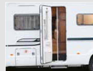
Entrance door Entrance door with secure 3-point locking, hidden hinges, double seal system and stepwell light
