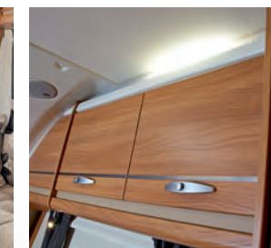
^^ Concealed low energy lighting over the lockers in the seating and bedroom areas
