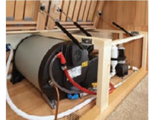
Dual fuel Truma combi boiler with en-route operation
