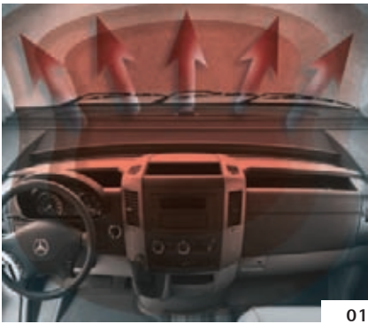
Instrument panel: Blower on the windscreen
