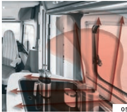
Kitchen: Hot air outlet at window
