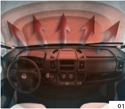
Instrument panel: Blower on the windscreen
