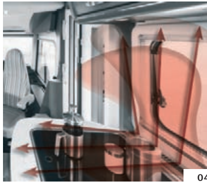
Kitchen: Hot air outlet at window
