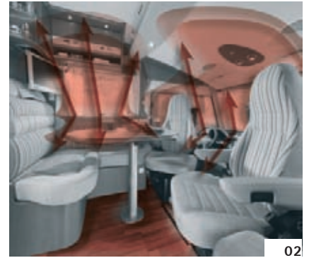
Living space: Hot air outlets at window and under the L-seating group
