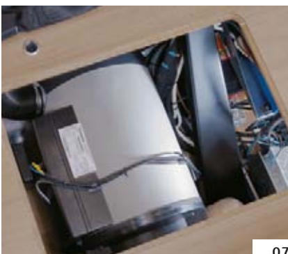
07 High heating power included: With 6.000 watts of power, the Truma Combi 6 heater, installed as standard, has no trouble bringing the temperature inside the vehicle up to a cosy level even when it is freezing outside. Thanks to its central location under the seating group, the heat is distributed optimally throughout the vehicle.
