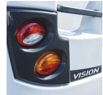
Light Cluster Incorporating twin fog lights and reversing lights.
