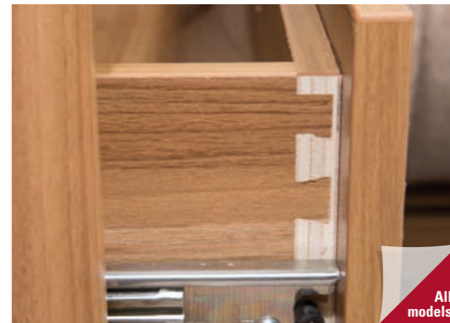
Craftsman-built cabinetry with dove-tailed drawers
