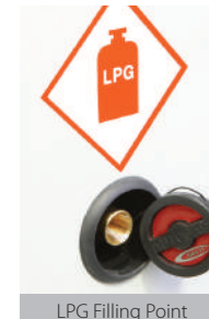
LPG Filling Point
