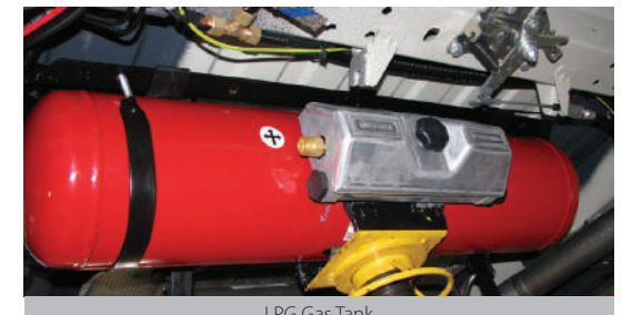
LPG Gas Tank
