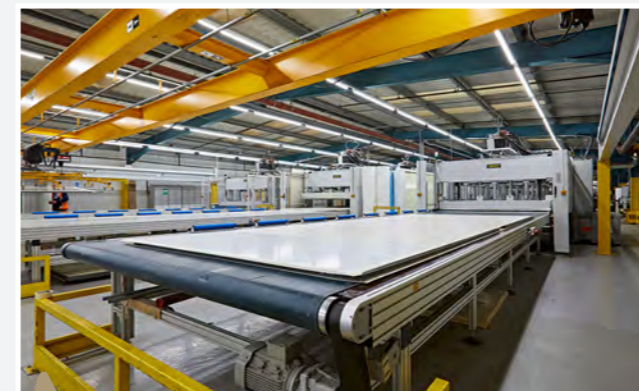
'SMART' GRP sidewall during the production process.
