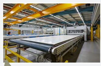
'SMART' GRP sidewall during the production process.
