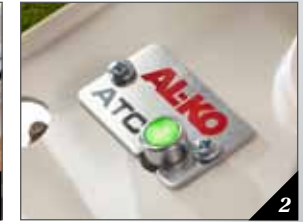
1) Polyplastic double glazed opening sunroof with night blind in front dome. 2) AL-KO ATC Trailer Control System.
