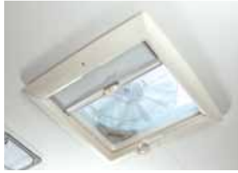
The ventilator/extractor skylight (Welcome version) allows extracting stale air and ventilating the inside very quickly.
