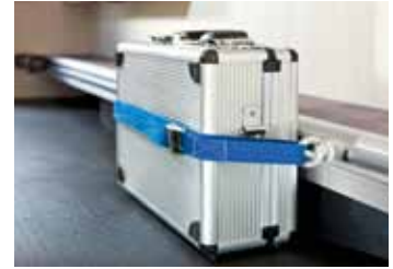
The hold has rails and attachment points for solidly attaching bikes or scooters (Welcome version).
