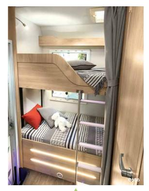
Low bed which can be folded to turn the storage compartment into a garage
