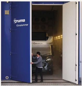
The EN1646-1 standard makes no compromises. To obtain the highest level (Grade 3), the standard requires that at an outside temperature of -15°C, the inside temperature must be able to reach +20°C in less than four hours.
