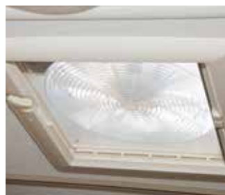
The three-speed Omnivent roof extractor fan takes care of steam from cooking
