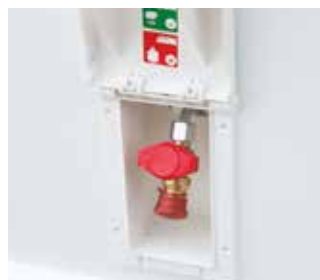
A barbecue point, so that you can take gas from your caravan cylinder to your barbecue
